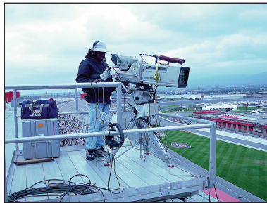
Figure 6.63 The Race/FX system is built on the systems that came before it. It uses the same modified pan/tilt head with one addition: A gyroscope measures the vibration that the camera undergoes so that any "bouncing" video produced by these cameras using a very long focal length lens is recorded. This movement is used by the graphics computers to add bounce to the onscreen graphics, so that the keyed information moves with everything else in the picture.
