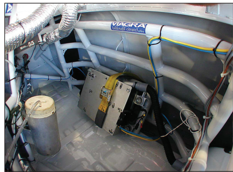
Figure 6.64 All the race cars used by the 43 NASCAR teams have this data acquisition and positioning system (DAPS) installed against the roll cage on the "passenger" side of the vehicle (left photo). The right photo shows the antenna mount for telemetry transmit and GPS receive. Each team has about 10 vehicles, set up to run at various tracks. Most teams take a couple cars to each race. The box collects telemetry such as throttle position, steering, fuel consumption, braking and speed, among other items. (Source: Sportvision/GPS World)
